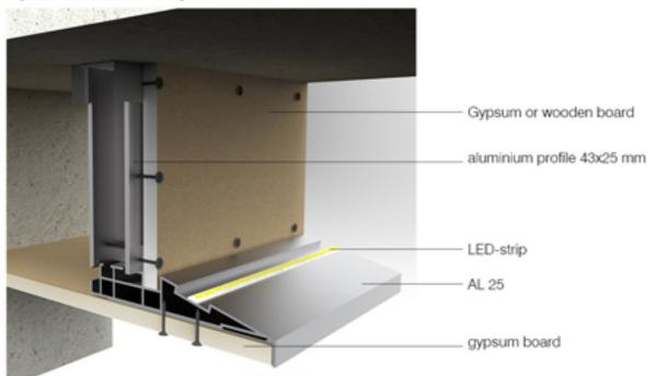
LED stripes can be placed directly on the profile in 15 degrees angle from the horizontal line. Outside the cornice you will see the 17mm wide white profile frame. The profile is 167,1mm wide and is available in 2,5m and 5m lenghts. AL25 profile minimum recommended fastening is after every 40cm with gypsum frames by using screws. It is also possible to add gypsum on top of the profile, to prevent the light accessing backside of the ceiling and to finish the cornice side.
